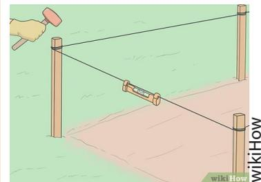
Measuring slope with string line level.
