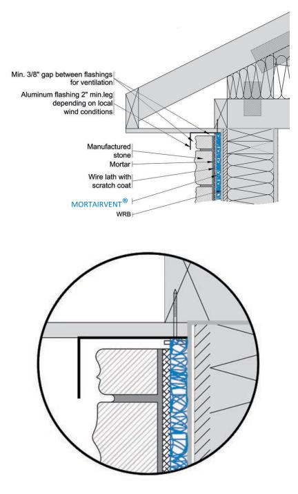
Be mindful of differential movement when the flashing is attached directly to the soffit.
