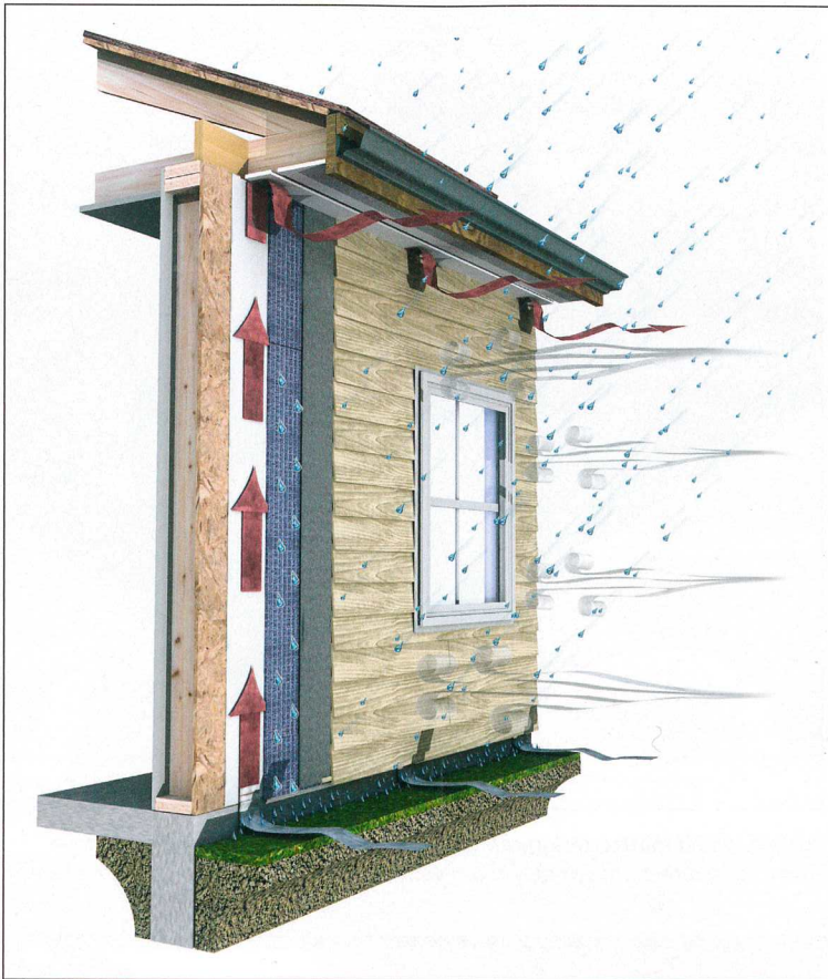
Installing a polymeric-engineered rainscreen behind the cladding allows for proper draining and drying within the wall system.
