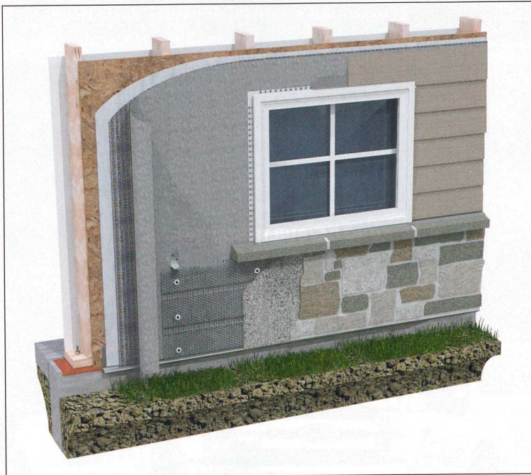
The rainscreen for multiple sidings with entangled net drainage and ventilation mat has a heat bonded filter fabric attached to one side.
