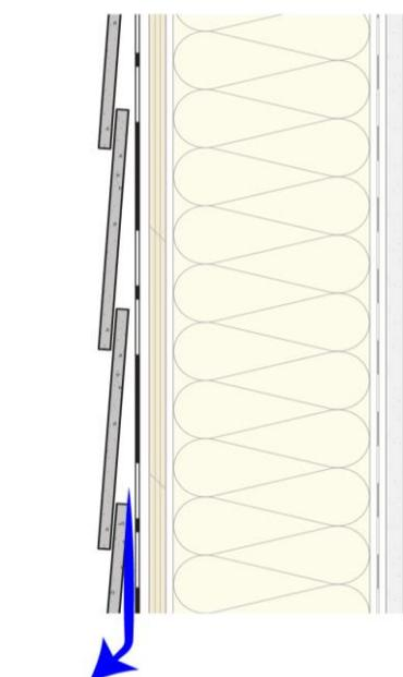
One layer of building paper with detailing for drainage under wood/fiber cement cladding
