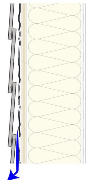
Textured wrap under wood/fiber cement cladding
