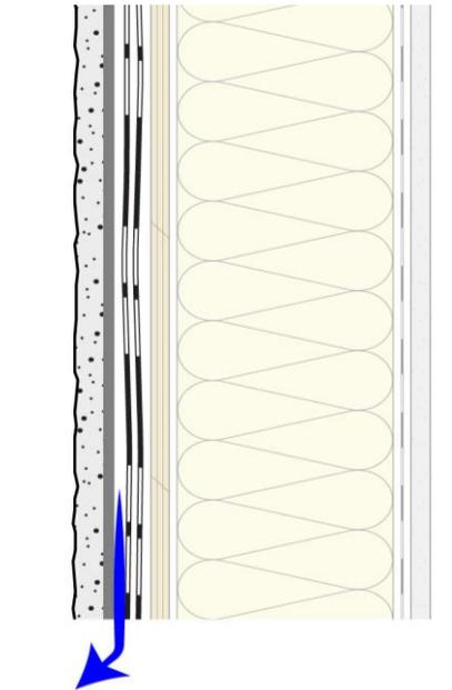
Two layers of building paper under stucco cladding
