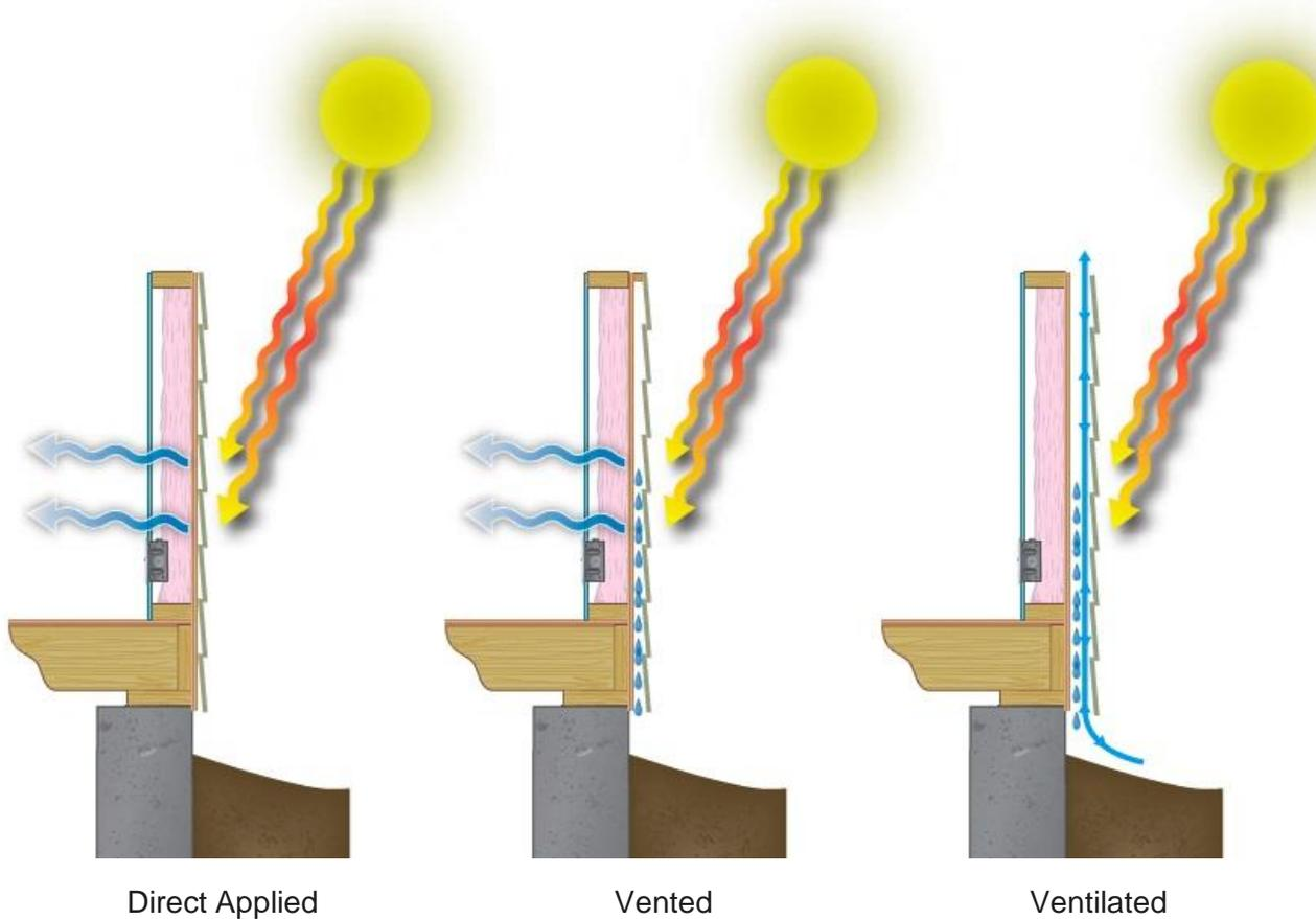
The three most common wall designs are direct applied, vented, and ventilated.
