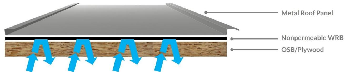
Roofing Felts | Building Paper | Ice and Water Membranes | Nonpermeable WRB
