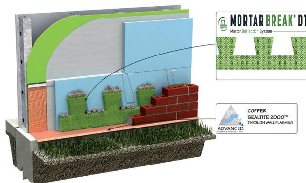
Mortar Break<sup>®</sup> DT is available in .4", 1" & 2" thicknesses
