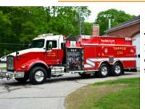
**Tanker 234 (T234)** is a 2017 US Tanker Heritage body on a Kenworth T800 Chassis. It has a 1,500 GPM Waterous pump, 3,000-gallon water tank, tanker shuttle equipment, as well as EMS and LifeStar landing equipment. Tanker 234 shuttles water to structure fires and is first due at LifeStar incidents.
