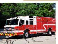
**Rescue 134 (R134)** is a 2013 Pierce Heavy Rescue. It features full EMS capabilities including AED, cold water rescue suits, 15 KW PTO powered generator, six hydraulic lines to include Amkus spreader, cutter and rams, pneumatic lift bags, cribbing, gas meters, 8,000-pound capacity winch, light tower and scene lights, and seating for six. Rescue 134 is first due to vehicle accidents or any incident where heavy rescue capabilities are needed.
