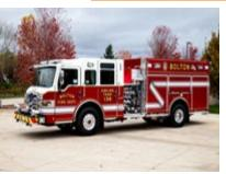
**Engine Tank 134 (ET134)** is a 2023 Pierce Velocity engine. It features a 1,500 GPM single-stage Hale pump, 1,000-gallon booster tank, foam equipment, thermal imaging camera, EMS equipment, and seating for six. Engine Tank 134 responds to vehicle accidents and fires and is second due to structure fires.
