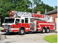
**Truck 134 (TK134)** is a 2008 Pierce 100-foot aluminum ladder truck on a Velocity chassis. The truck has a 2,000 GPM pump, 500-gallon booster tank, thermal imaging camera, 15 KW generator, 6,000 watts of lighting, Amkus extrication equipment including hydraulic cutter and spreader, EMS equipment, and seating for six. Truck 134 is first due at structure fires.
