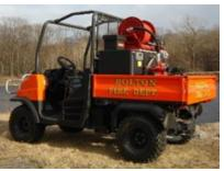
**Utility Vehicle 134 (UTV134),** a 2004 Kubota RTV900, complements Forestry 134 for wildland firefighting and remote search and rescue operations. It is equipped with detachable firefighting or EMS equipment packages.
