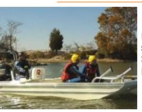
**Marine 134 (M134)** is a 2020 Rescue One 16-foot aluminum boat with a 40 HP 4 stroke engine, center console, and has a dive/rescue platform. It is a trailer towed by Service 234. Our boat has seen service not only in Bolton Lake but in many lakes and ponds in eastern Connecticut.
