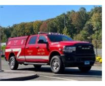
**Service 134 (S134)** is 2021 Dodge Ram 3500. It has full EMS capabilities including AED, equipment for command operations, and has seating for five. Service 134 is used to transport LifeStar crews and is first due to house medical calls.
