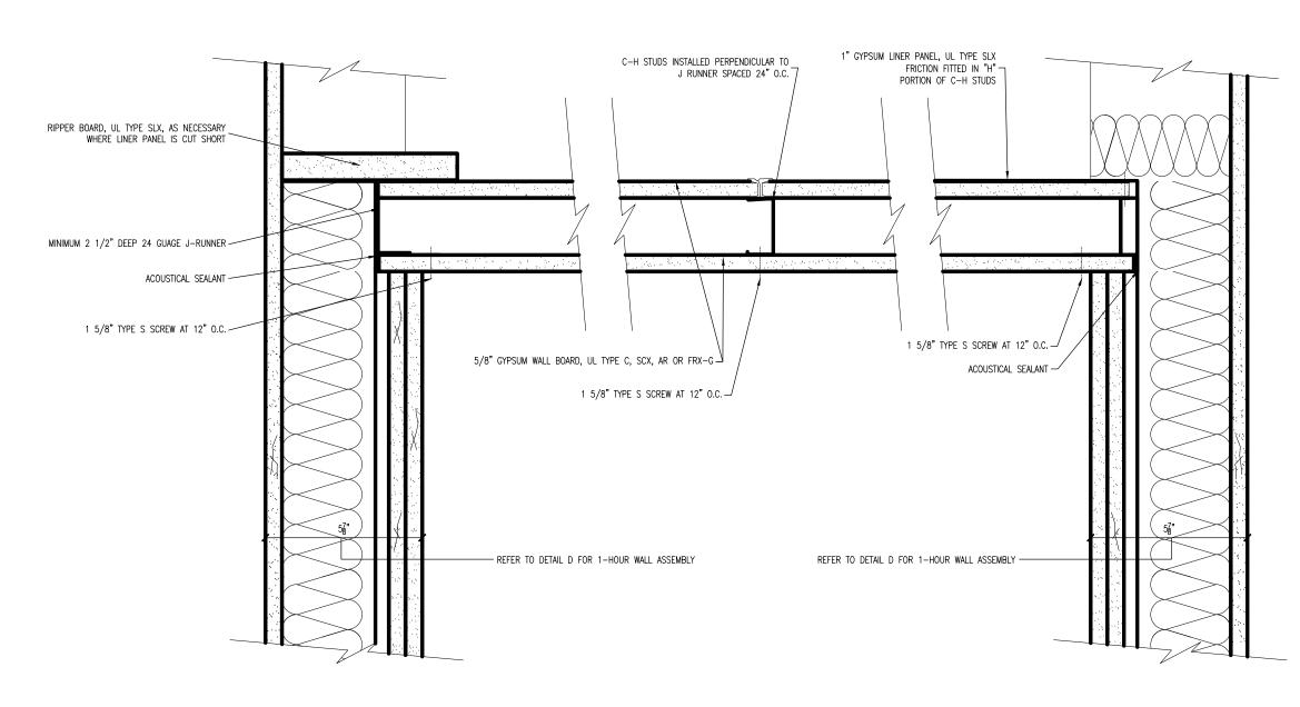
**15** SHAFT WALL/CEILING DETAIL SCALE: 3" = 1'-0"
