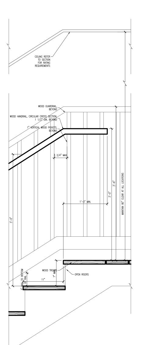
**19** TOP OF EXTERIOR COMMON STAIR DETAIL SCALE: 1 1/2" = 1'-0"
