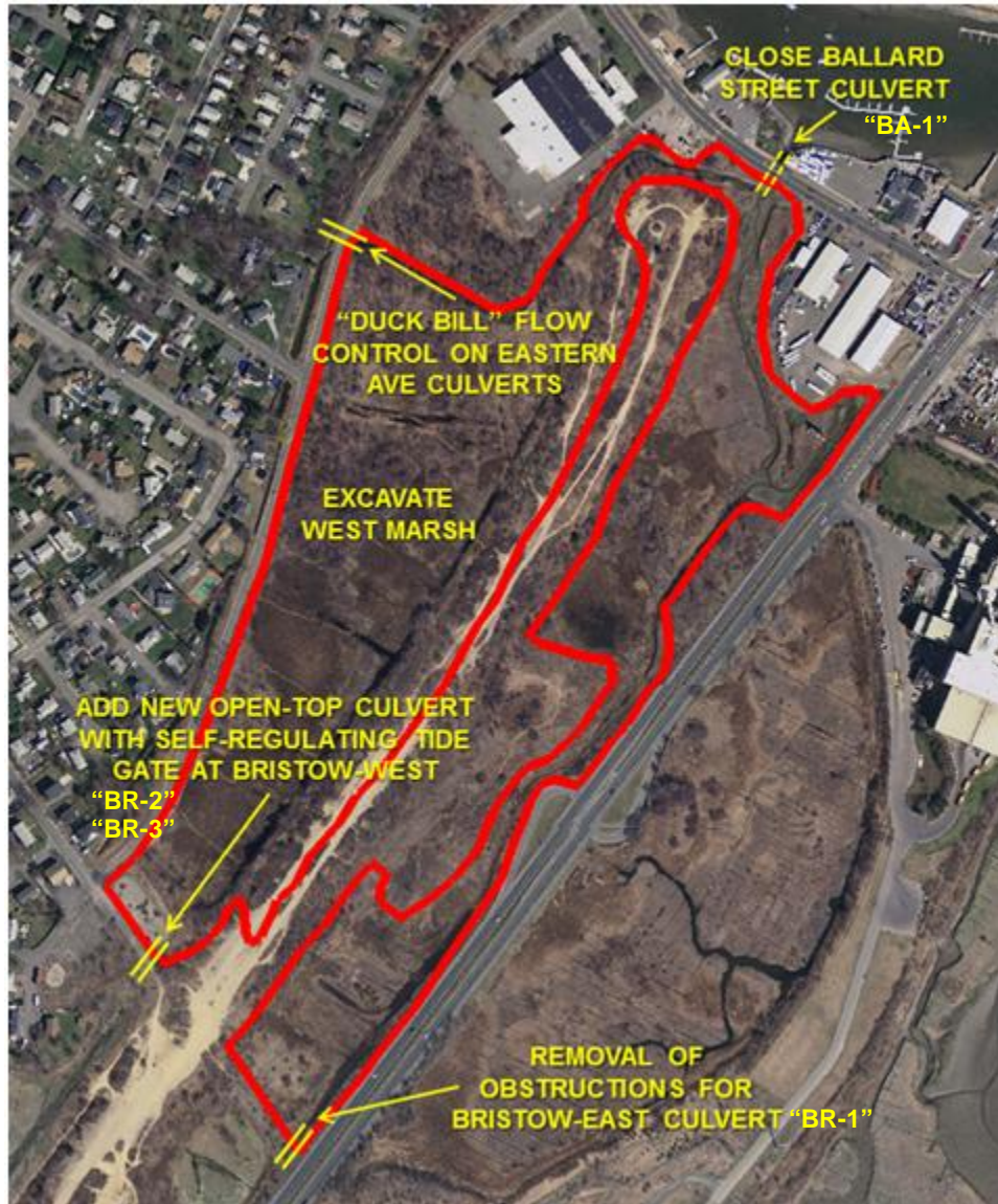
Fig. 3.03 Alternative 3 with SRT at Bristow (“BR-2” and “BR-3”) and Ballard Street Closed
