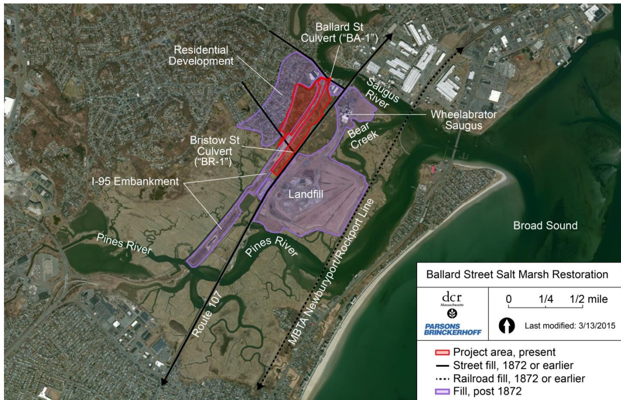
Fig. 1.08 Fill placement since 1872
