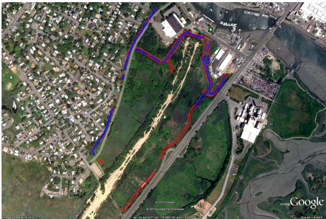
Figure 4-18. Contours of tidal maximum (red) and minimum (blue) water surface elevation during normal tides for existing conditions. Disconnects in the water surface elevation contours represent culverts and/or areas that are shallow water.
