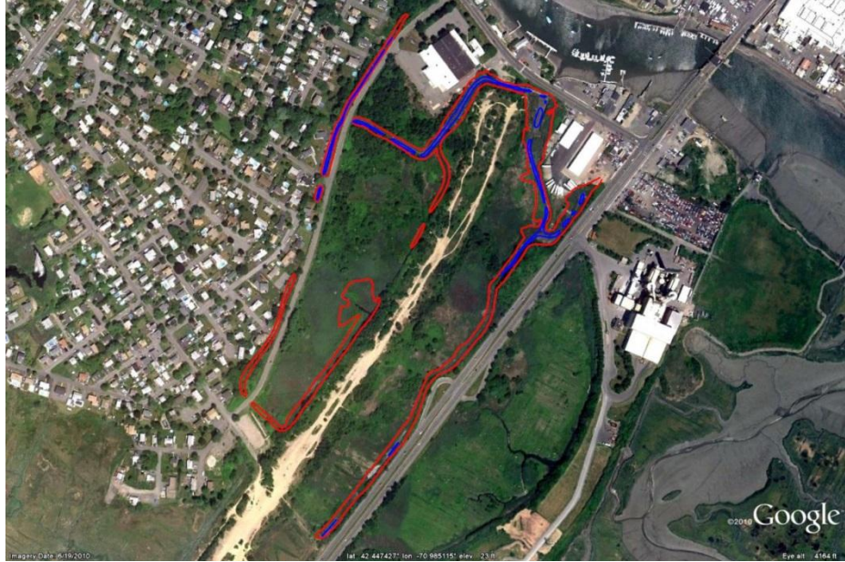
Figure 5-18. Contours of maximum (red) and minimum (blue) water surface elevation during normal tides, new Ballard Street tide gate alternative. Disconnects in the water surface elevation contours represent culverts and/or areas of shallow water.
