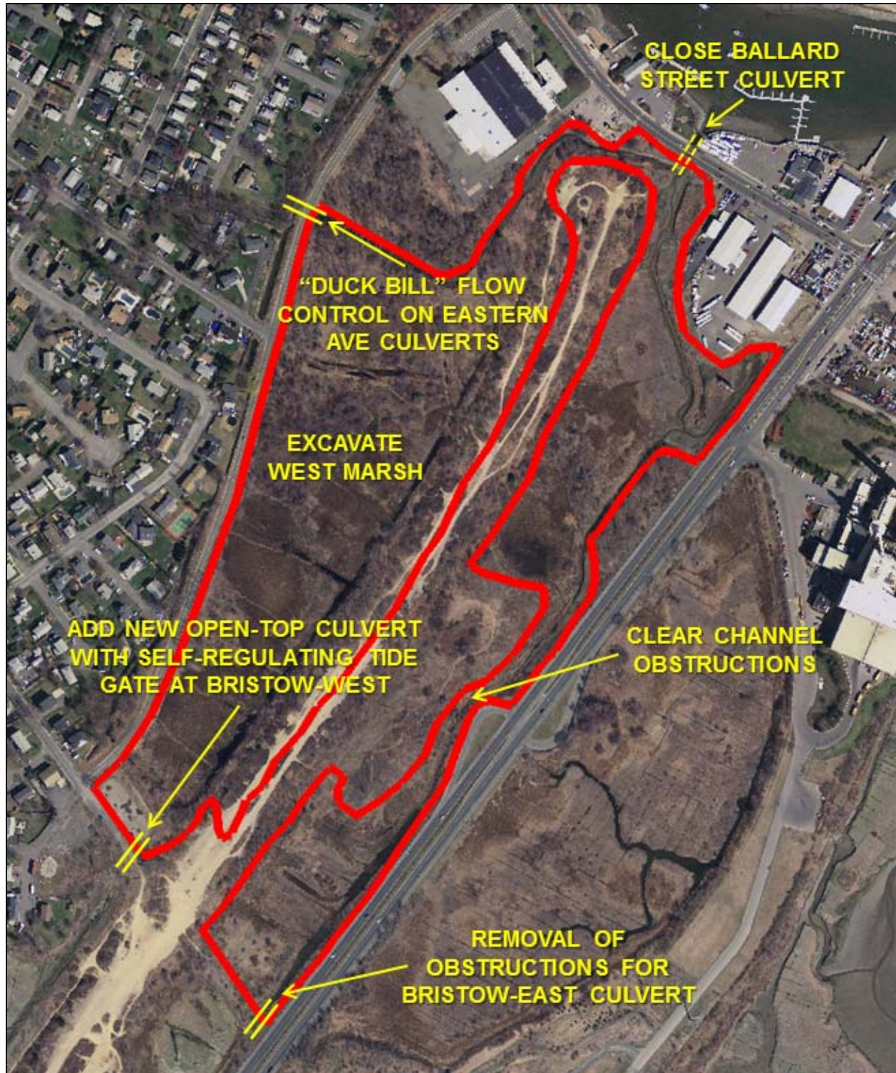
Figure 5. Schematic representation of Alternative 3, Install New SRT at Bristow-West and Close Ballard Street Culvert, where the hydraulic connection to the marsh system is through the Bristow-East and Bristow-West culverts. Only moderate lowering of the western marsh is required to achieve restoration design goals. The area outlined in red represents the hydrodynamic model domain and is not intended to represent tidal inundation area.
