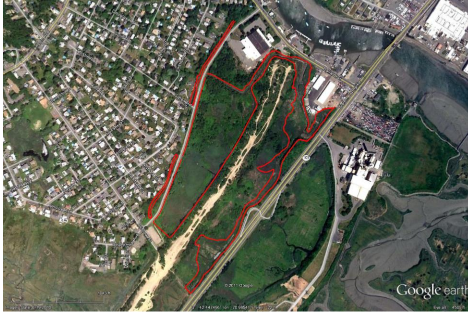
Figure 5-33. Maximum extent of inundation during normal tides (full spring to neap tidal cycle) for the modified NRCS alternative.
