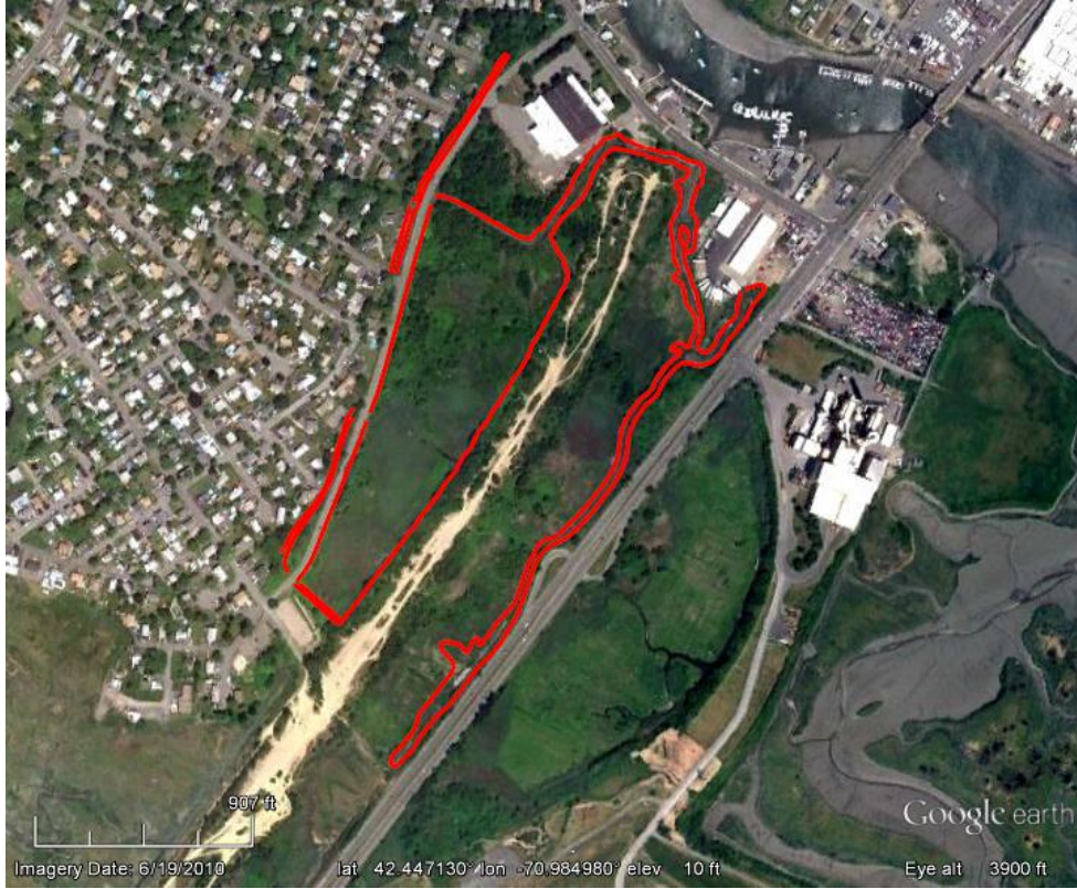
Figure 6-10. Maximum water surface contour (approximately equivalent to the monthly high spring tide) for the updated refined alternative.
