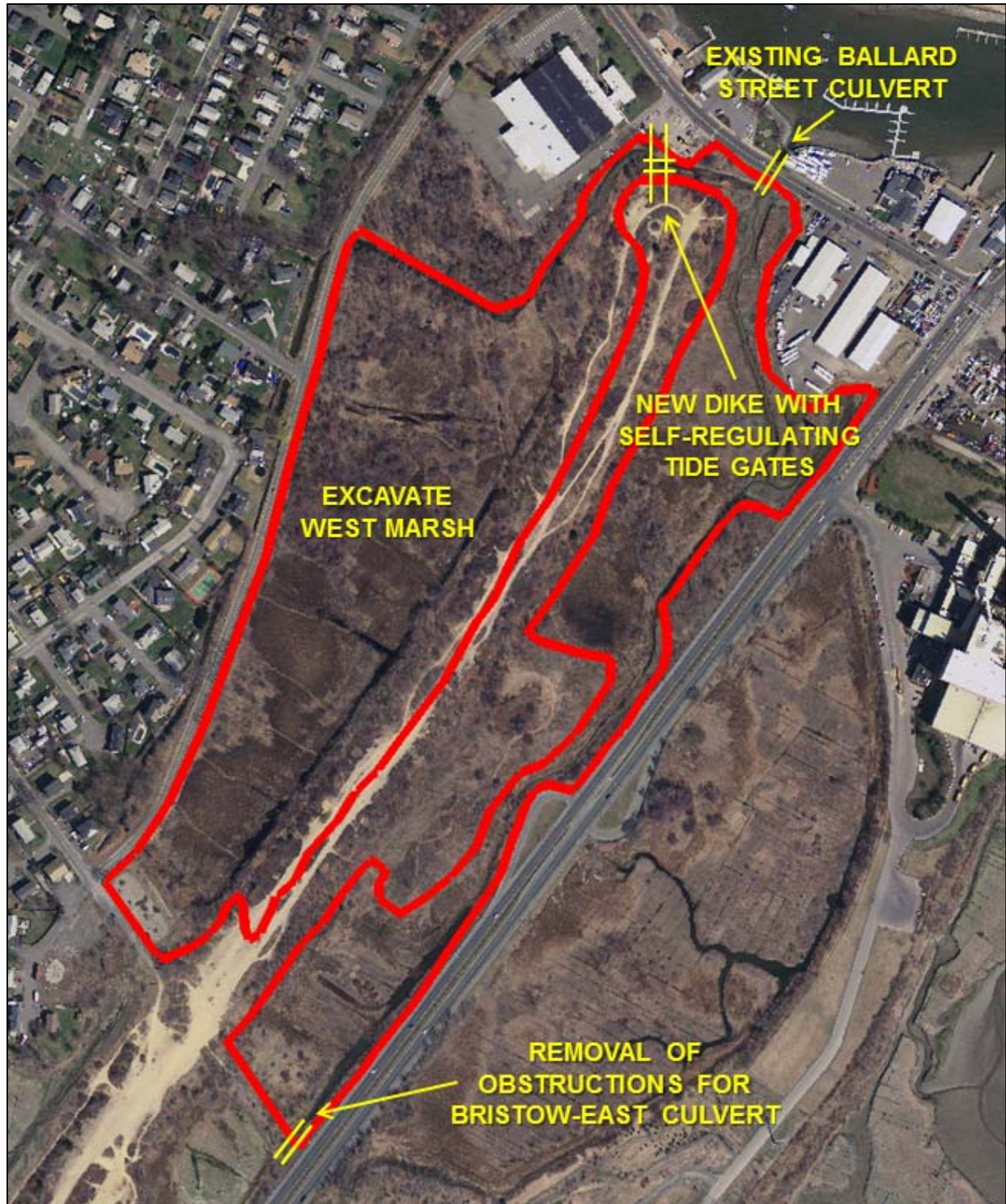
Figure 4. Schematic representation of Alternative 2, Modified NRCS Design, where the hydraulic connection for the Ballard Street salt marsh system is primarily through the existing 4-ft diameter culvert with the flap gate removed and an additional connection is provided by removing obstructions at the Bristow-East culvert. Substantial lowering of the west marsh and installation of SRTs to further attenuate the tide signal is required to achieve design goals. The area outlined in red represents the hydrodynamic model domain and is not intended to represent tidal inundation area.
