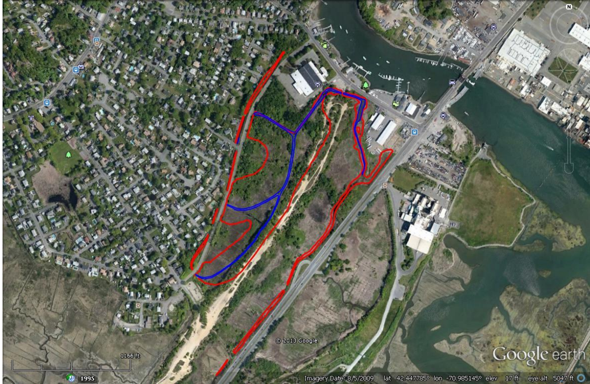
Figure 7-9. Contours of mean high water (red) and mean low water (blue) water surface elevation during normal tides, preferred alternative.
