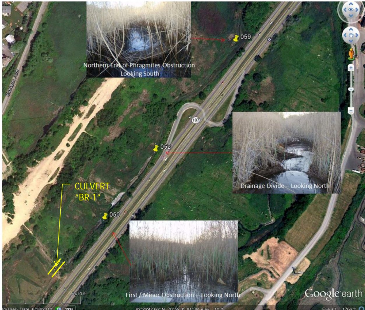
Fig. 2.27: Obstructions in Pines Channel (Eastern Channel) North of Bristow Street East Culvert (“BR-1”) (Source: Woods Hole Group, Inc., 2013, Fig. 6-3 – See Appendix 1)
