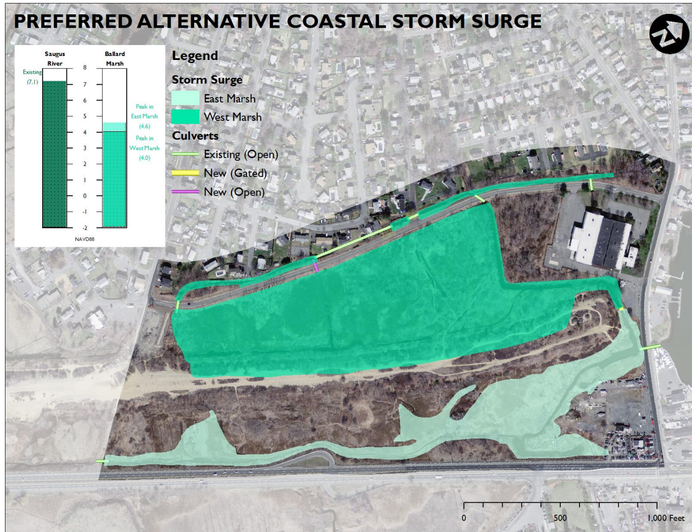
Figure 7-12. Graphical representation of water levels within the Ballard Street marsh system for storm surge conditions (results from model simulation) with the preferred alternative in place.
