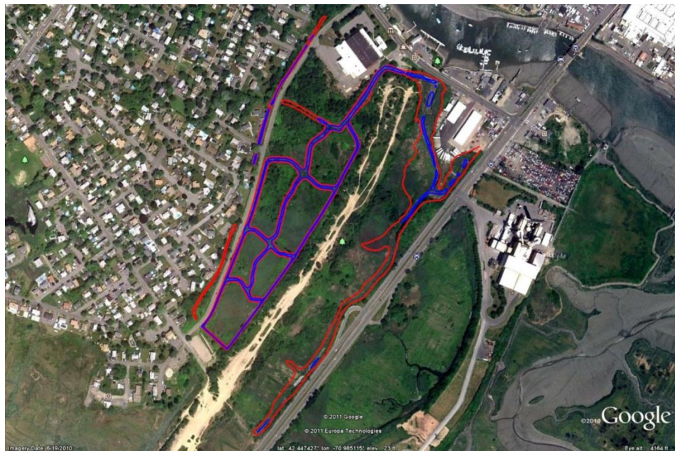
Figure 5-6. Contours of maximum (red) and minimum (blue) water surface elevation during normal tides, preliminary NRCS alternative.
