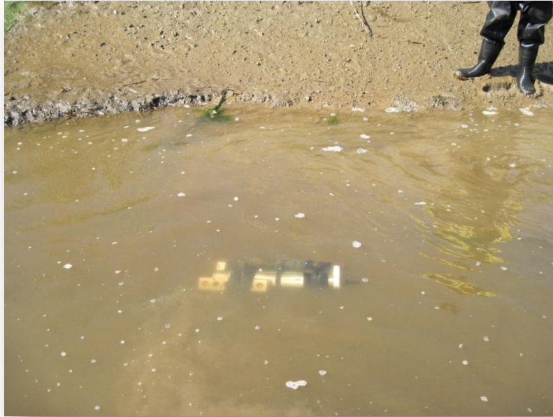
Figure 2-3. Seabird Electronics SBE37 Microcat deployed in Ballard St. marsh.
