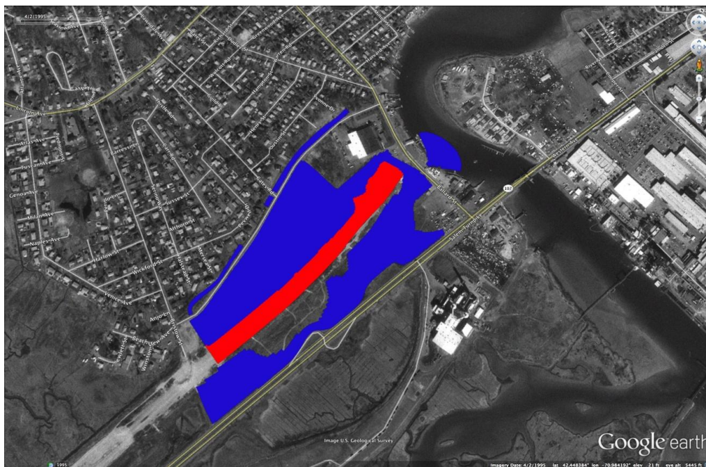
Figure 7-1. Original model domain (blue) with expanded domain area (red) for DCR extraction alternatives.
