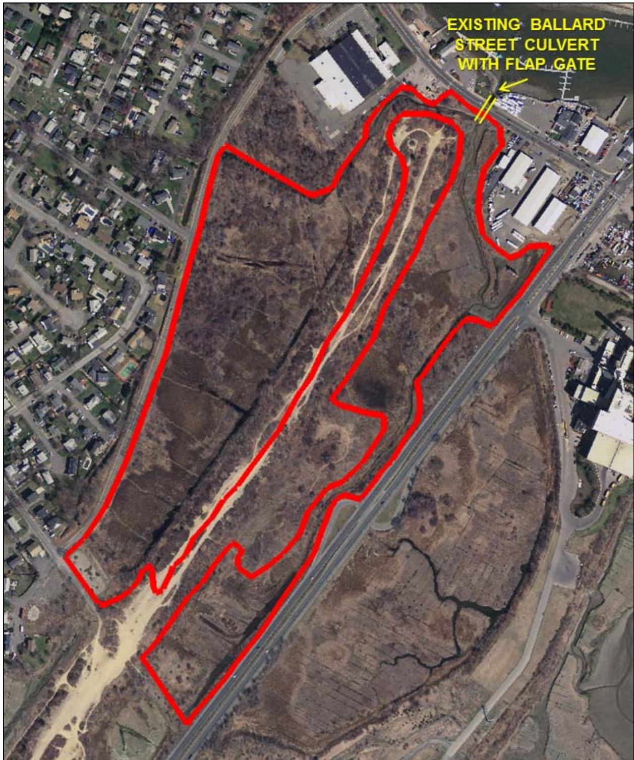
Figure 3. Schematic representation of Alternative 1, Existing Conditions, where the only hydraulic connection for the Ballard Street salt marsh system is the existing 4-ft diameter culvert with the flap gate connecting to the Saugus River. The area outlined in red represents the hydrodynamic model domain and is not intended to represent tidal inundation area.
