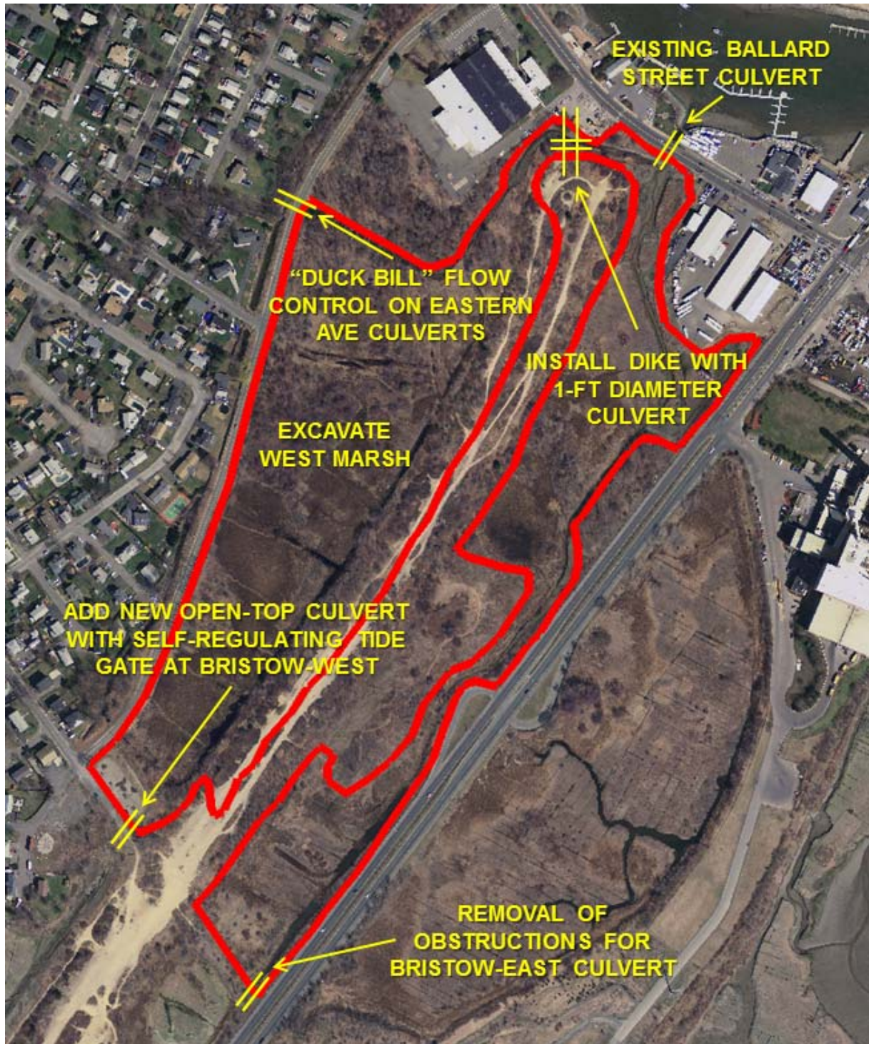
Figure 6. Schematic representation of Alternative 4, Install New SRT at Bristow-West and Install Dike in Channel near Ballard Street with 1-ft Culvert through Dike, where the hydraulic connection to the western marsh is primarily through the Bristow-West culvert and the hydraulic connections to the eastern marsh is via both the Ballard Street and Bristow East culverts. Only moderate lowering of the western marsh is required to achieve restoration design goals. The area outlined in red represents the hydrodynamic model domain and is not intended to represent tidal inundation area.
