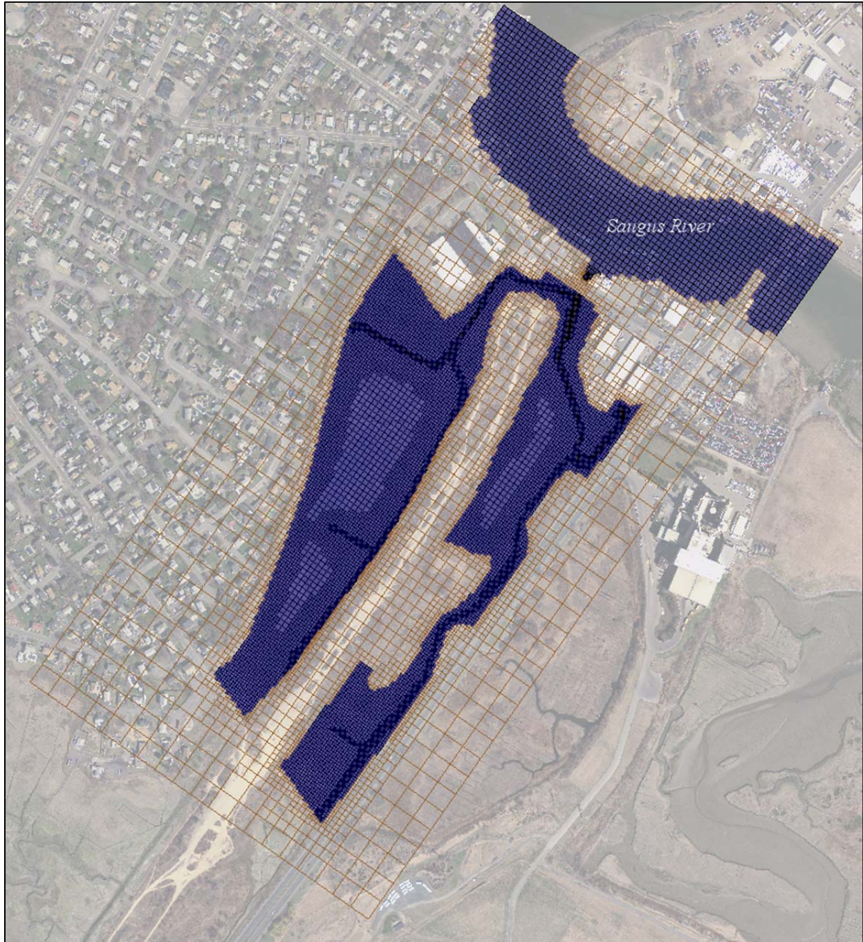
Figure 10. CMS telescoping mesh developed for existing conditions at Saugus Marsh. Blue shaded area indicates active computational cells, while unshaded cells are inactive during runs of the model.
