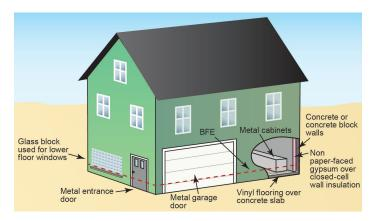
Figure 7: Flood damage-resistant materials
