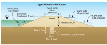
Figure 10: Residential levee and typical levee cross section
