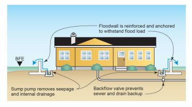
Figure 9: Residential floodwall
