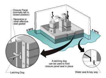
Figure 6: Detail of floodproofed building utility
