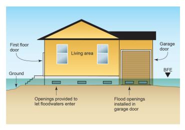
Figure 4: Flood openings and their placement
