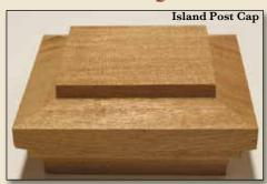
**★ Post Cap Finial Care ★**PREPARATION... All Nantucket Post Cap finials are constructed of quality laminated clear Redwood and Western Red Cedar. They should be sealed BEFORE installation with an oil base primer, paint, stain or preservative to ensure long life. These should be applied to all surfaces INCLUDING the base.
