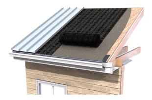
Creating an air space or gap between the roof sheathing material and a metal roof (or a wood shingle roof), separates the roofing materials which reduces conduction of heat. This also allows convective cooling of the roof by means of air movement through the air gap. This air gap is commonly referred to as above sheathing ventilation (ASV). During cold weather the
